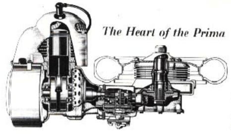
The new Prima has a fourspeed-pearbox and you change gears with a footgedal. If you want to change gear, just touch the pedal gently – and the gear is changed. From the gear box the power goes to the rear wheel by way of the drive shaft which is running in an oil both.
